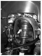
11. Remove the two spring strut assembly lower mounting nuts.
