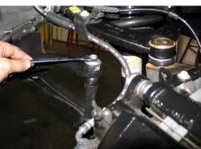
13. Once all the mounts have been un-bolted, hold the spindle assembly while slightly pushing down, dislodging the bottom spring/ strut assembly from its lower mounts. Carefully remove the entire spring/strut assembly from its perch, paying extra attention to not damage or over extend brake hoses.
